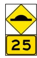
PW-39 HUMP SIGN WITH, PW-25 ADVISORY SPEED SIGN (25KM/HR)
